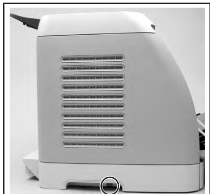
Figure 1. Removing the left side cover screw (circled).
